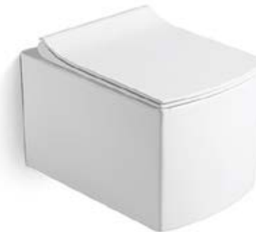
WH-036 Wall-hung toilet Size: 510x350x360 mm P-trap, 180mm roughing-in
