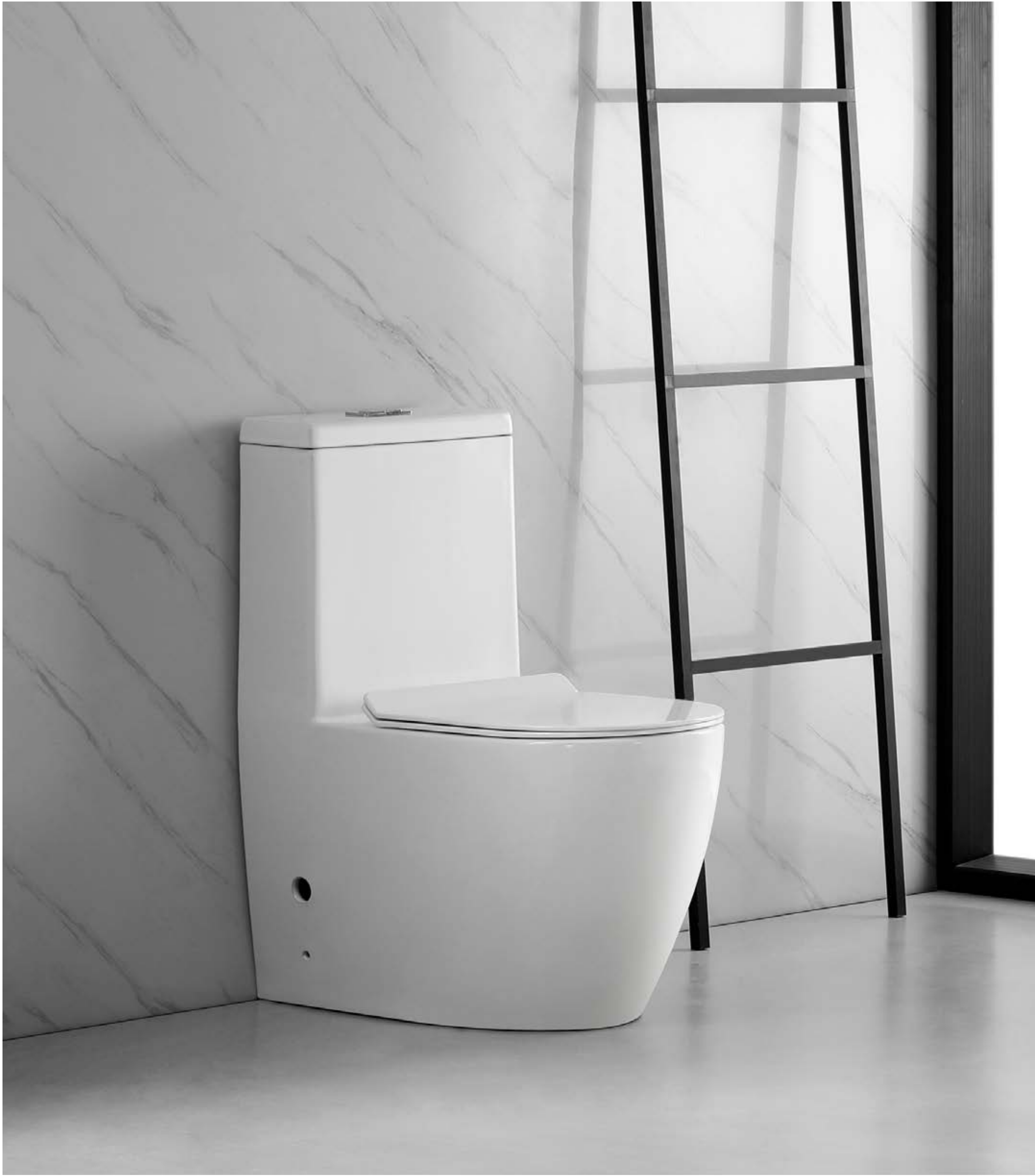
8022 Washdown one-piece toilet Size: 720x375x810 mm P-trap, 180 mm roughing-in S-trap, 250 mm roughing-in
