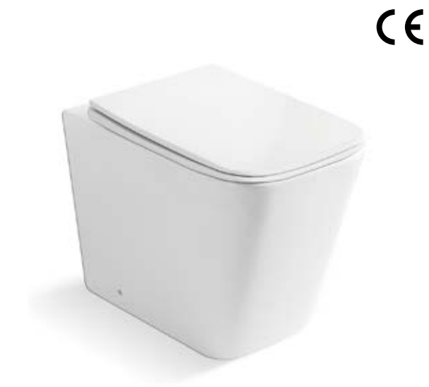
1048FW Washdown floor mounted toilet Size: 555x360x400 mm P-trap, 180 mm roughing-in
