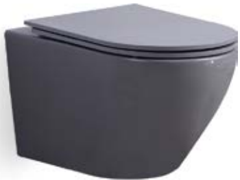
WH-003GM Wall-hung toilet Size: 485x365x370 mm 535x365x350 mm P-trap, 180 mm roughing-in Color: Grey Matt
