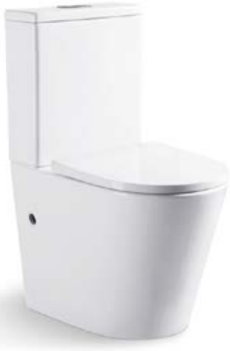
1046A Washdown two-piece toilet Size:690x370x820 mm P-trap,180mm roughing-in
