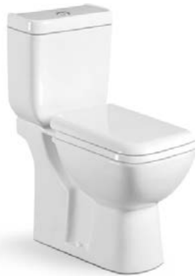
1036A Washdown two-piece toilet Size: 680x380x800 mm P-trap, 180mm roughing-in S-trap, 250mm roughing-in
