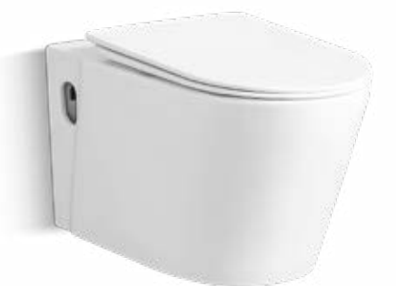
WH-018 Wall-hung toilet Size: 570x360x340 mm P-trap, 180mm roughing-in
