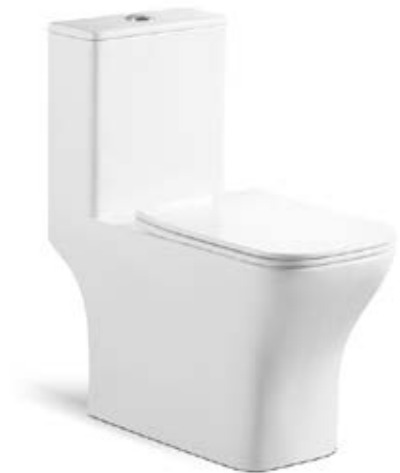
8217 Washdown one-piece toilet Size: 665x350x750 mm P-trap, 180mm roughing-in S-trap, 250mm roughing-in
